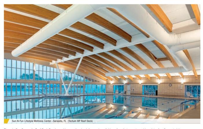
Three-in-One Composite Roof Deck Panels provide acoustics, insulation, and a nailable surface that accepts a wide variety of roofing materials.
